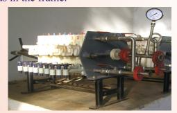
In the recessed type, the slurry is fed through the central inlet and the solids are retained in the recess between the plates, while the filtrate is collected through the corners.
